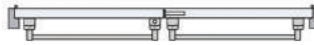
Pair of non-rebated Doors with one Vertical Device and one Mortise Lock Device
