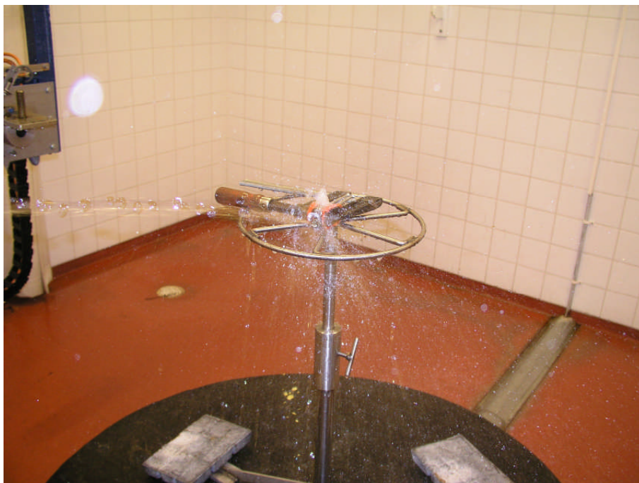
Electronic cylinder during spray test, IPX5
