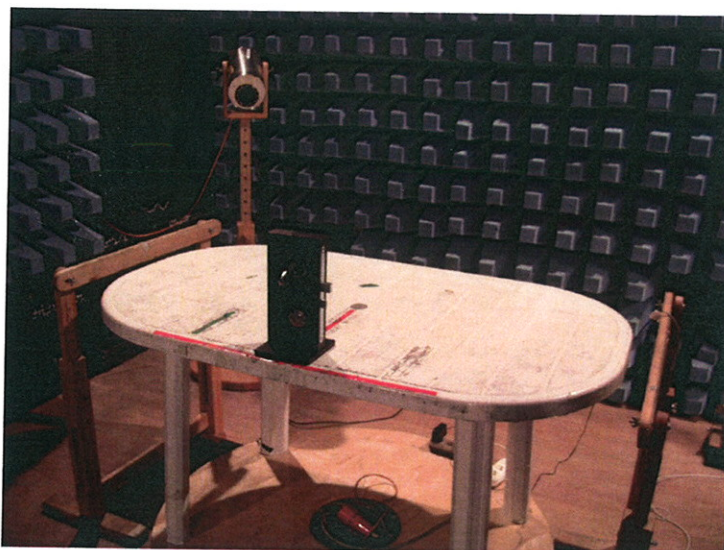
Photo of the test set-up during the radiated electromagnetic field immunity test.
