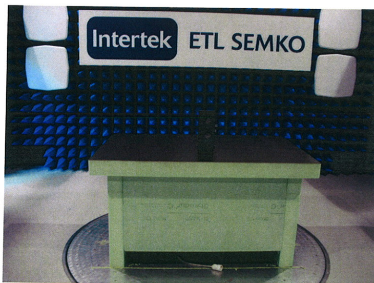
Photo of test set-up during the radiated emission test
