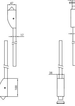
Panic Exit Devices Rim version PED/GL Lateral rod device length: 1100 mm PED/GL
