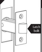
Insert latch with the curved side of the latch bolt facing in the direction that the door closes.
