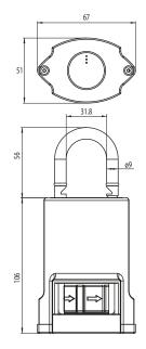
It is very important to push the shackle firmly when closing this will guarantee the padlock is correctly sealed
