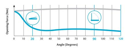
Typical symmetric rack-and-pinion with guide rail
