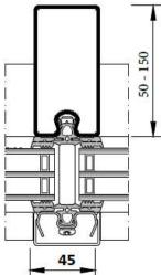
Thermfix Vario is the system for thermally insulated, internal and external grade, curtain walls and skylights comprising of mild steel profiles, stainless steel pressure plates and aluminium or stainless-steel cover caps.
